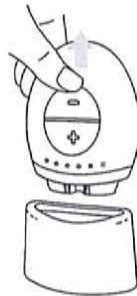
Figure 4: Remove or leave the base unit in the charger.
