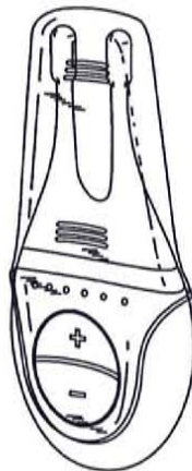
Figure 10: Cover attached to base unit to protect disposable tip.
